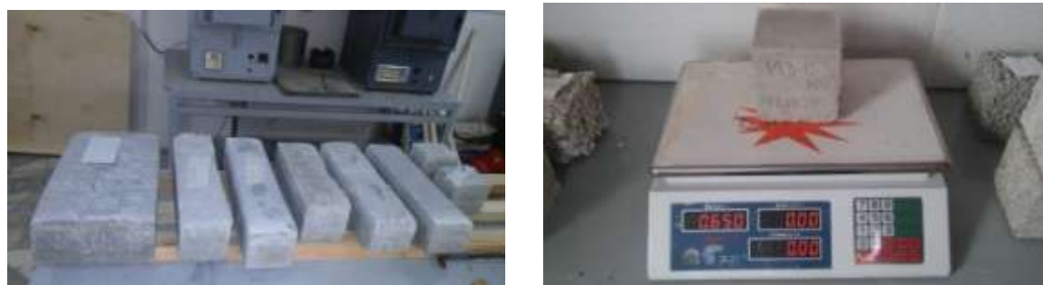
Figure 2. Fibrogazobeton samples prepared for testing
